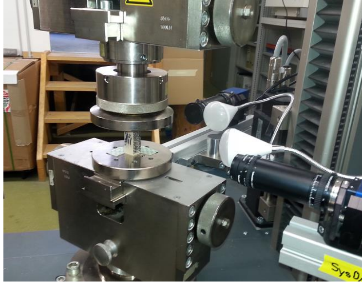
Figure 1. Compression test set up.
